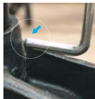
If the pointer stick is in a different position, the result is the hub needing to be replaced. If the pointer stick fails to reach the suspension, the problem is with the shock absorber.
