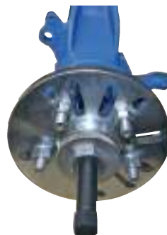
Drive shaft extraction from hub
