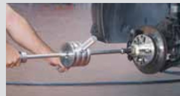
Pulling out the wheel hub, using a slide hammer, optional code GO520 (optional)
