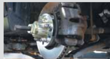
Pushing out the drive shaft, mechanically using the tool set
