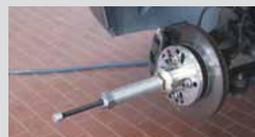
Pushing out the drive shaft, using a 16-Ton mechatronic screw, optional code GO1016
