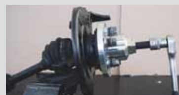
Pushing out the drive shaft, mechanically on the workbench
